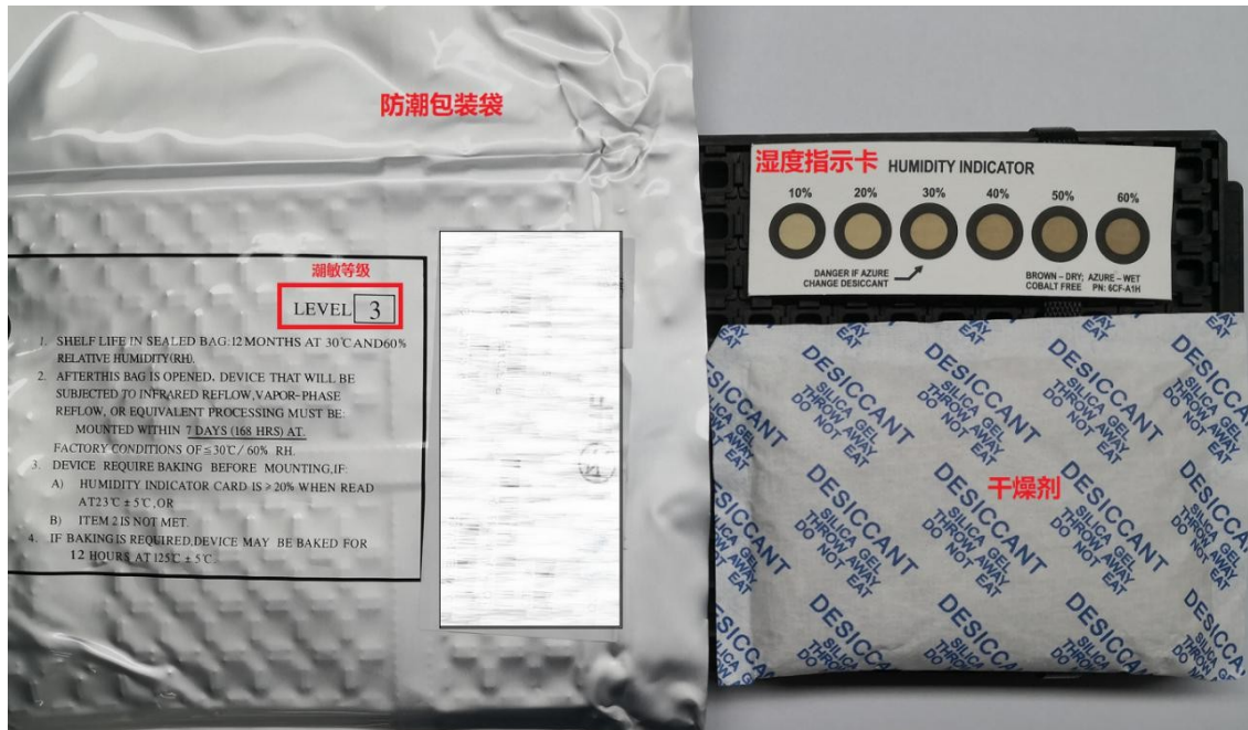
Figure 4-2 Schematic diagram of dry vacuum packaging materials
